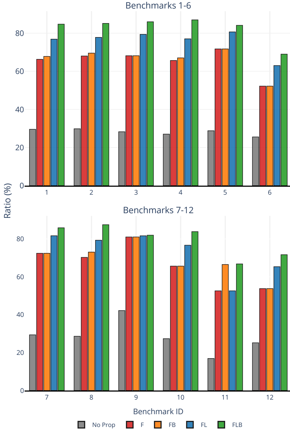
Figure 3.7: Effect of forward (F), lateral (L), and backward (B) propagation on sparsity ratios of einsum benchmarks with 50% input sparsity. The y-axis is average sparsity across all tensors in the benchmark. The higher the bars, the better, as more sparsity is discovered in the computational graph.
